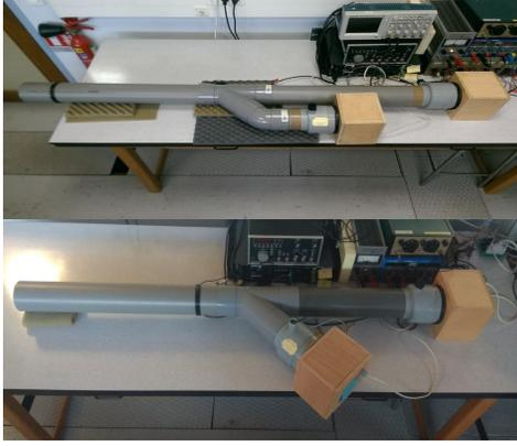
Fig. 2: Duct active noise control test bench - Configuration Go (top), configuration G (bottom)
