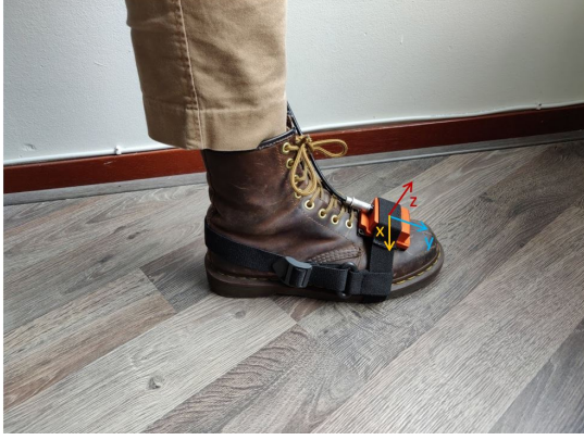
Fig. 2. Experimental setup with foot-mounted sensor.
