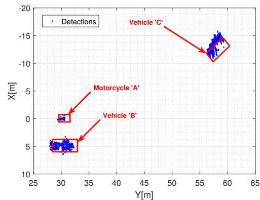
Fig. 13. Detection points in cartesian plane for the proposed method. Red rectangles depict the approximated ground truth.
