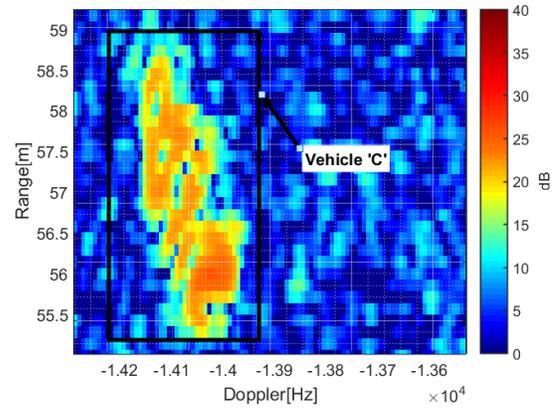
Fig. 12. Range-Doppler spectrum of the proposed method, zoomed in on around vehicle 'C'.
