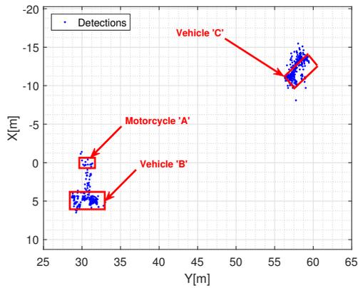
Fig. 10. Detection points in cartesian plane for integration time of 50 msec. Red boxes mark the approximate true object position.
