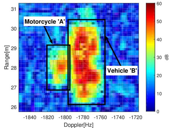
Fig. 5. Range-Doppler spectrum obtained for integration time of 300msec, zoomed in on Motorcycle 'A' and Vehicle 'B' bins.
