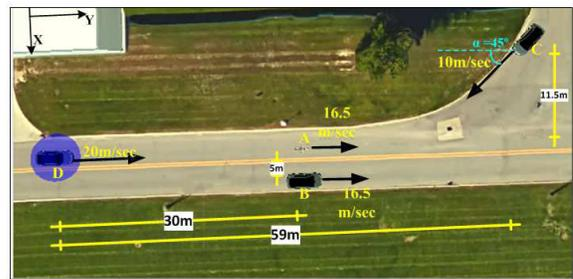
Fig. 4. Bird-eye view of tested scene. Objects, distances and velocities direction and magnitude are marked on the figure. Test radar mounted on front bumper of vehicle 'D'.
