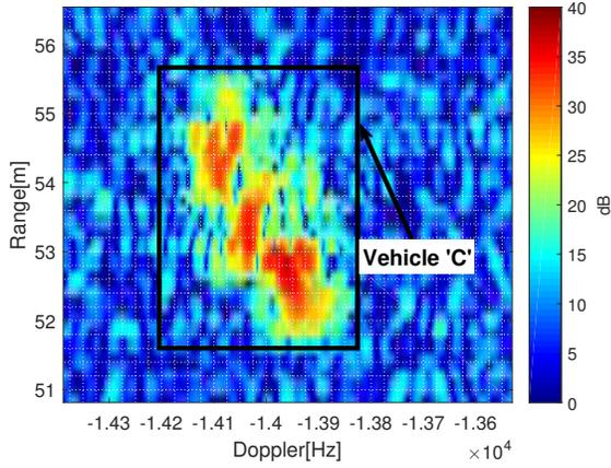
Fig. 6. Range-Doppler spectrum obtained for integration time of 300msec, zoomed in on vehicle 'C' bins.
