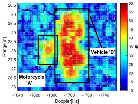
Fig. 11. Range-Doppler spectrum obtained of the proposed method, zoomed in on Motorcycle 'A' and vehicle 'B'.
