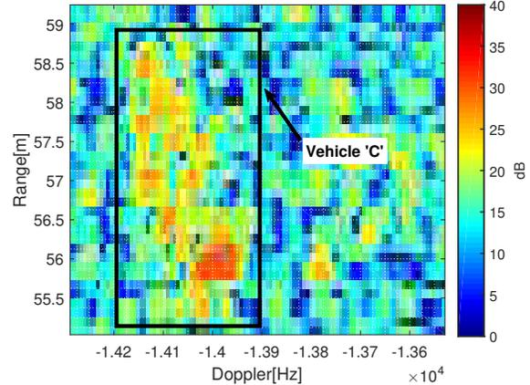
Fig. 9. Range-Doppler spectrum obtained for integration time of 50msec, zoom in on vehicle 'C' bins.
