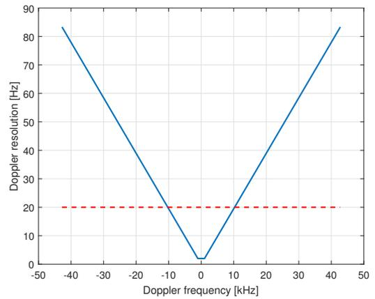
Fig. 3. Doppler resolution vs. Doppler frequency
