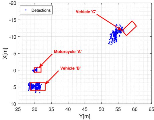
Fig. 7. Detection points in cartesian plane for integration time of 300msec. Red boxes mark the approximate the true object position.
