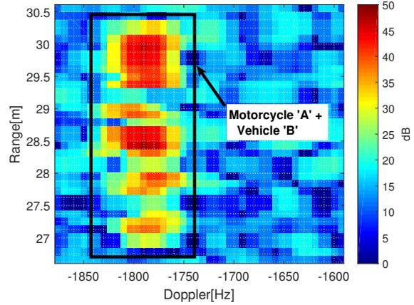
Fig. 8. Range-Doppler spectrum obtained for integration time of 50msec, zoomed in on Motorcycle 'A' and Vehicle 'B' bins.
