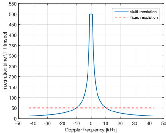
Fig. 2. Integration time vs. Doppler frequency
