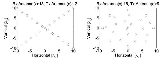
Fig. 3. Mills Cross array (left), curvilinear array (right)
