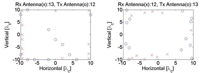
Fig. 2. Array design obtained with initially uniform antenna configuration (left), Array design obtained with initially random antenna configuration (right).
