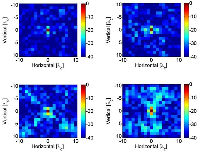
Fig. 4. Two dimensional reconstruction results in dB: for the design obtained with initially uniform array (upper left), for the design obtained with initially uniform array (upper right), for Mills cross array (bottom left), for curvilinear array (bottom right)
