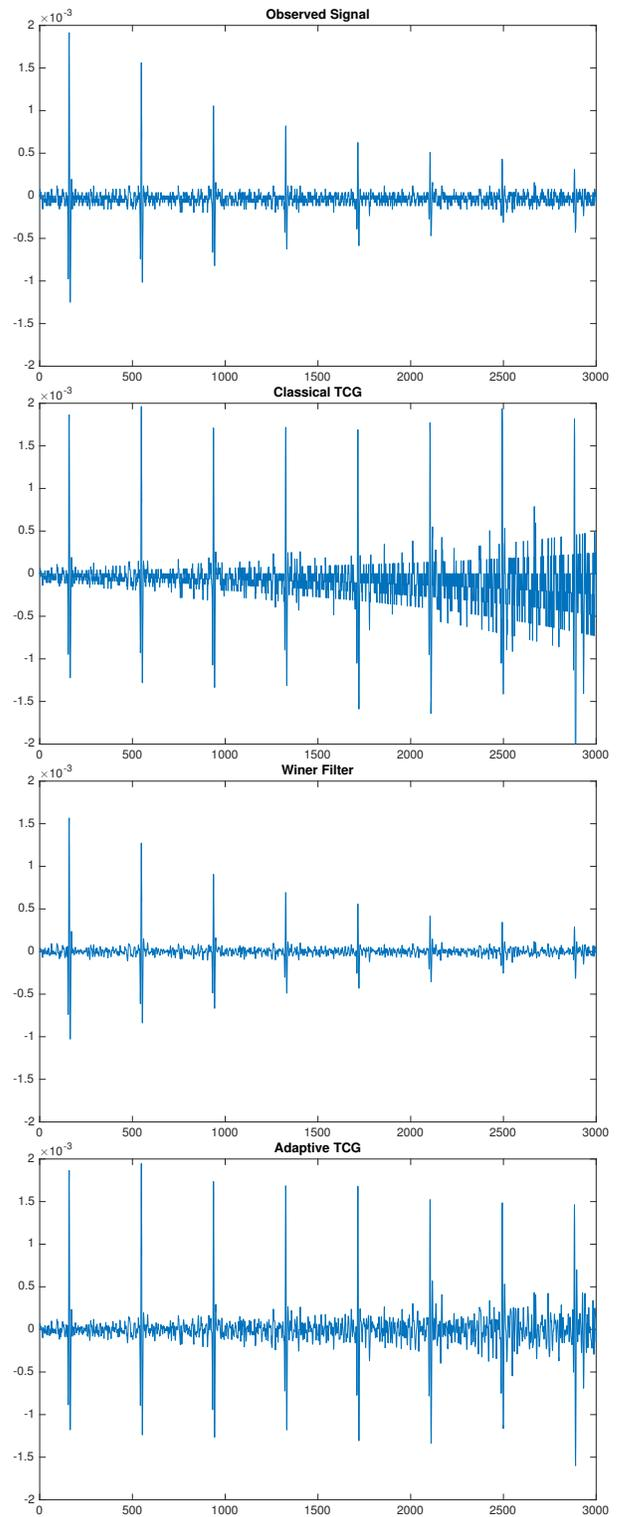
Fig. 3. Experimental results for Classical TCG, Wiener filter and the proposed Adaptive TCG. The proposed method was capable of correcting the amplitudes of the echoes and increasing SNR at the same time.
