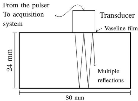
Fig. 2. Depiction of the experimental setup. Due to multiple reflections of the ultrasound wave in the aluminum block, the excitation burst is received by the transducer as several echoes. Subsequent echoes have smaller amplitudes, which are inversely proportional to the distance traveled by the ultrasound beam.
