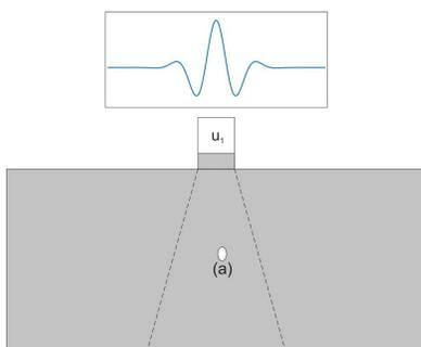
Figure 1. Defect detection with Ultrasound Testing
