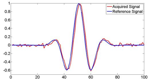
Figure 2. The acquired signal is subject to white gaussian noise and a subsample time delay
