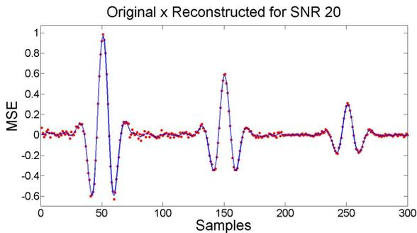
Figure 4. MSE between the generic continuous signal and the reconstructed signal. In red we have the acquired data, and in blue we have the reconstructed signal from the last iteration.
