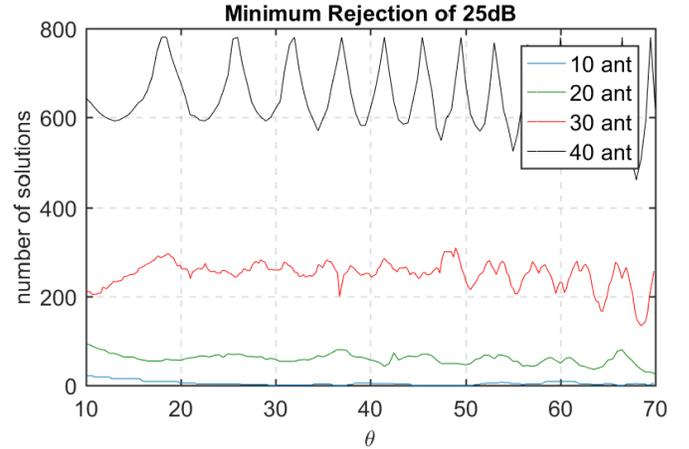
Fig. 2. Number of useful radiation patterns with minimum rejection of 25 dB versus angle ( $\theta \in [10^\circ, 70^\circ]$ , main beam at  $\theta_{max} = 90^\circ$ ) and for different size of antenna array, blue for 8 elements out of 10, green for 18 out of 20, red for 28 out of 30 and black for 38 out of 40.
