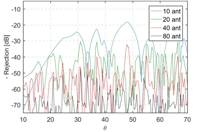
Fig. 1. Opposite of maximum rejection of interference in [dB] (relative to the main lobe level) versus angle ( $\theta \in [10^\circ, 70^\circ]$ , main beam at  $\theta_{max} = 90^\circ$ ) for different size of antenna array, blue for 8 elements out of 10, green for 18 out of 20, red for 38 out of 40 and black for 78 out of 80.
