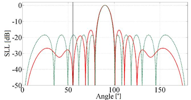
Fig. 6. Result of the optimization for low SLL, stable beamwidth and maximum rejection at  $\theta = 55^\circ$  (see constraints in Tab. I) choosing 4 instantaneous patterns from the database TMA (see Fig. 4 and Fig. 5). In red the time-average pattern of optimal solution and in green for reference a Chebyshev pattern at -18.5 dB of SLL
