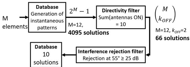
Fig. 4. Example of how a database is built by applying filters. Considering an antenna array of 12 elements: constant directivity of 10 elements ON, minimum rejection of 25 dB at  $\theta = 55^\circ$ .
