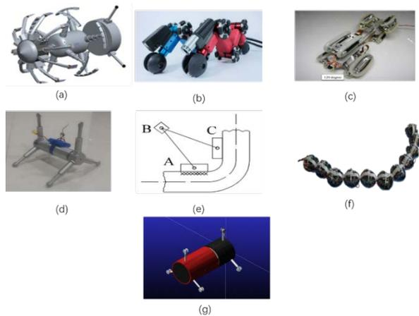
Figure 3. (a) The pig type [19], (b)The wheel type [20], (c) The track type [21], (d) The legged type [22], (e) The inchworm type [23], (f) The snake type [24], (g) The screw type [25].
