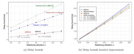
Figure 2: Parameter set: weights =  $\{4, 6, 7, 10\}$ ,  $l^{\min} = \{4096, 3072, 4608, 3072\}$  bits,  $l^{\max} = \{8704, 5632, 6656, 8192\}$  bits, burst sizes =  $\{30208, 19968, 24576, 27648\}$  bits, arrival rates =  $\{0.65, 0.85, 0.95, 0.55\}$  Mbit/s.
