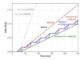
Figure 1: Service curve. Parameter set: weights =  $\{4,6,7,10\}$ ,  $l^{\min}$  =  $\{4096,3072,4608,3072\}$  bits,  $l^{\max}$  =  $\{8704,5632,6656,8192\}$  bits, burst sizes =  $\{30208,19968,24576,27648\}$  bits, arrival rates =  $\{0.65,0.85,0.95,0.55\}$  Mbit/s, server rate C = 5 Mbit/s.
