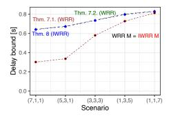
Figure 3: For the parameter description of traffic classes, we use the notation {low, mid, high, foi}: weights =  $\{4, 5, 6, 5\}$ , burst sizes =  $\{70, 700, 7000, 3000\}$  Kbit. We use the packet lengths  $l_i^{\min} = 576$  bytes,  $l_i^{\max} = 1500$  bytes and arrival rates = 7 Mb/s for each flow and a server utilization = 0.7.
