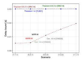
Figure 3: For the parameter description of traffic classes, we use the notation {low, mid, high, foi}: weights =  $\{4, 5, 6, 5\}$ , burst sizes =  $\{70, 700, 7000, 3000\}$  Kbit. We use the packet lengths  $l_i^{\min} = 576$  bytes,  $l_i^{\max} = 1500$  bytes and arrival rates = 7 Mb/s for each flow and a stabilizing utilization u = 0.7.
