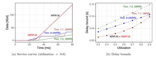
Figure 2: Parameter set: weights =  $\{4,6,7,10\}$ ,  $l^{\min} = \{4096,3072,4608,3072\}$  bits,  $l^{\max} = \{8704,5632,6656,8192\}$  bits, burst sizes =  $\{30208,19968,24576,27648\}$  bits, arrival rates =  $\{0.65,0.85,0.95,0.55\}$  Mbit/s.
