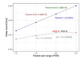
Figure 4: Impact of packet size range on the delay bounds. We choose the same parameters setting as in the previous experiment, except for the minimum packet size  $l_i^{\min}$ ,  $i = 1, \ldots, n$ .
