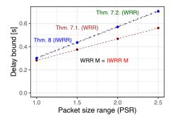
Figure 4: Impact of the packet size range on the delay bounds. We choose the same parameters setting as in the previous experiment, except for the minimum packet size  $l_i^{\min}$ , i = 1, ..., n.
