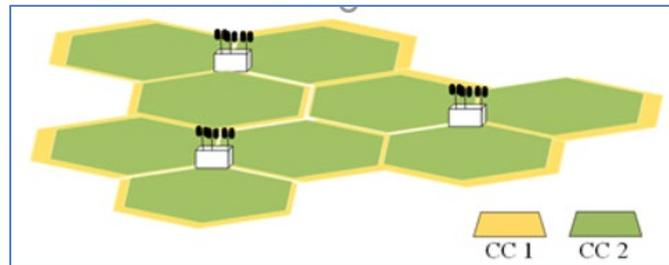
**Figure 3.** Carrier Aggregation Deployment in the same Macrocell
