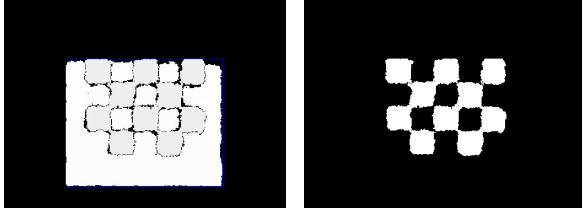
Figure 5: Left: 3D checkerboard target blob. Right: Binary image I_T .
