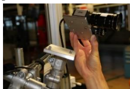
Figure 5: Camera dismantling with pinned fitting.
