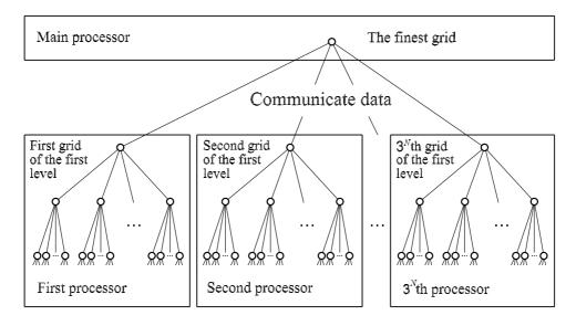
Fig. 1.2. Coarse grid distribution between the processors
