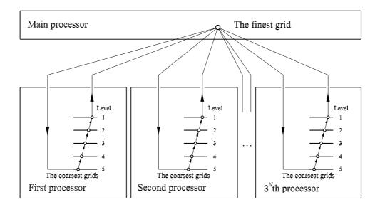
Fig. 1.3. Incomplete parallelization of the multigrid iteration
