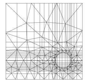
Fig. 2.4. Initial triangulation and auxiliary structured grid
