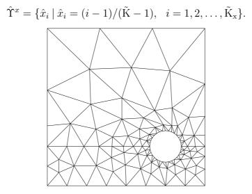
Fig. 2.1. Example of initial triangulation
