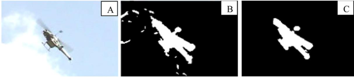
**Fig. 2 A. Original image, B. Processed image with noise from clouds, C. Processed image with optimized values of  $\alpha$  and  $\gamma$ .**
