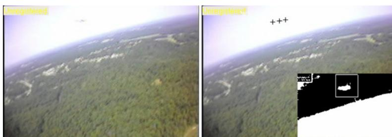
Fig. 4 Intensity saturation caused by the camera pointing to near the sun can cause noisy results.
