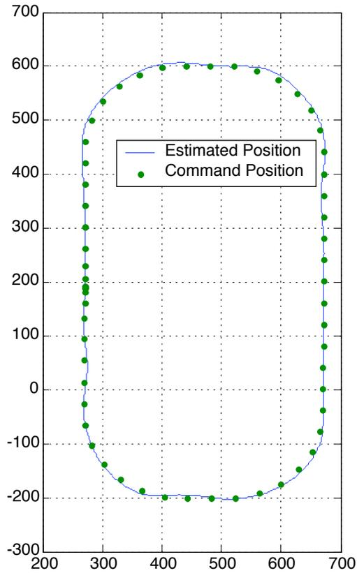
Fig. 8 Racetrack pattern flown at 40 ft/s starting and finishing in hover, commanded position plotted once per second
