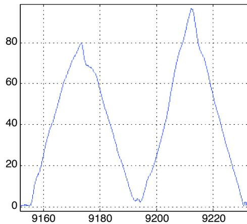
Fig. 9 Speed trial, first upwind (left) then downwind (right); speed limited by saturating collective upwind on first leg.
