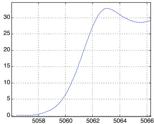
**Fig. 10 Recorded altitude during an automatic takeoff and climb to a hover at 30 ft of altitude.**
