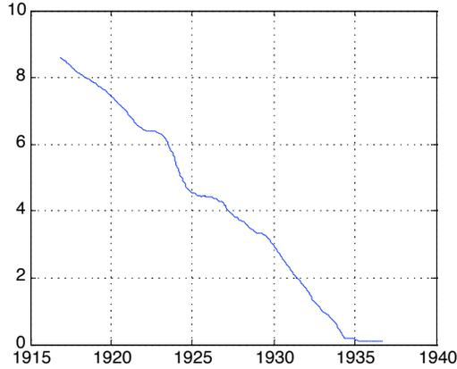
**Fig. 11 Recorded altitude during an automatic landing, after a descent at 0.5 ft/s.**
