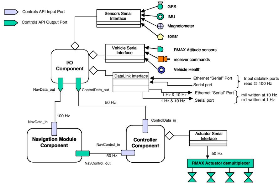
**Fig. 7 Open Control Platform (OCP) implementation of baseline GTMax guidance, navigation, flight control, and communication.**
