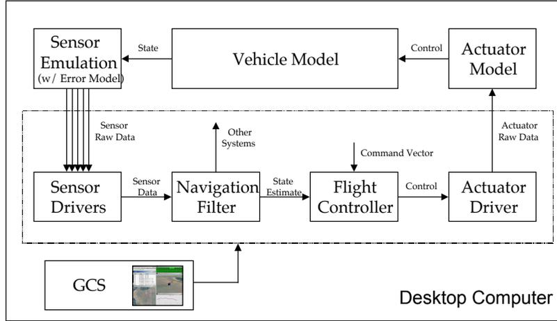
Fig. 5 Nominal software in the loop configuration.
