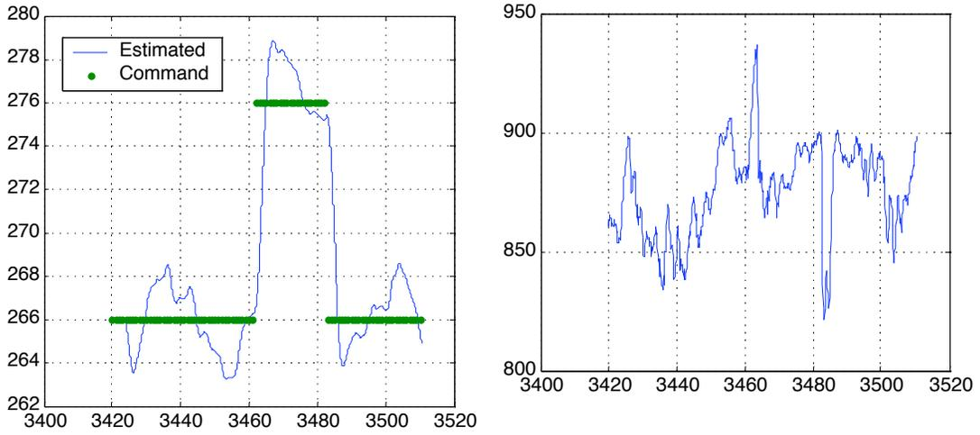
**Fig. 13 Utilizing rotor rpm to accommodate a simulated stuck collective actuator, step responses; (left) altitude and altitude command, (right) measured rotor rpm; note transient in rpm during climb and descent.**
