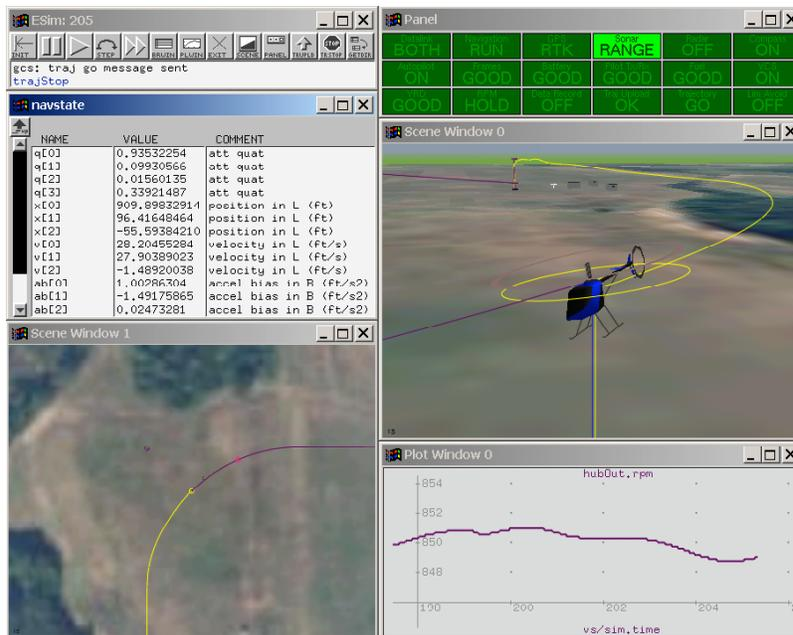
Fig. 4 Simulator scene generator and its use as a part of the Ground Control Station (GCS) operator interface.
