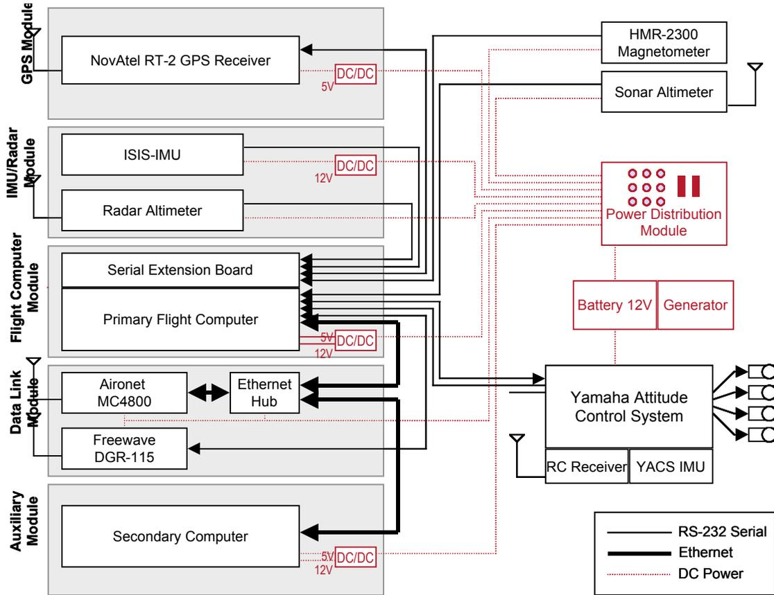
**Fig. 3 GTMax wiring diagram, including separation into modules, each with their own power regulation, air-cooling, and EMI shielding**
