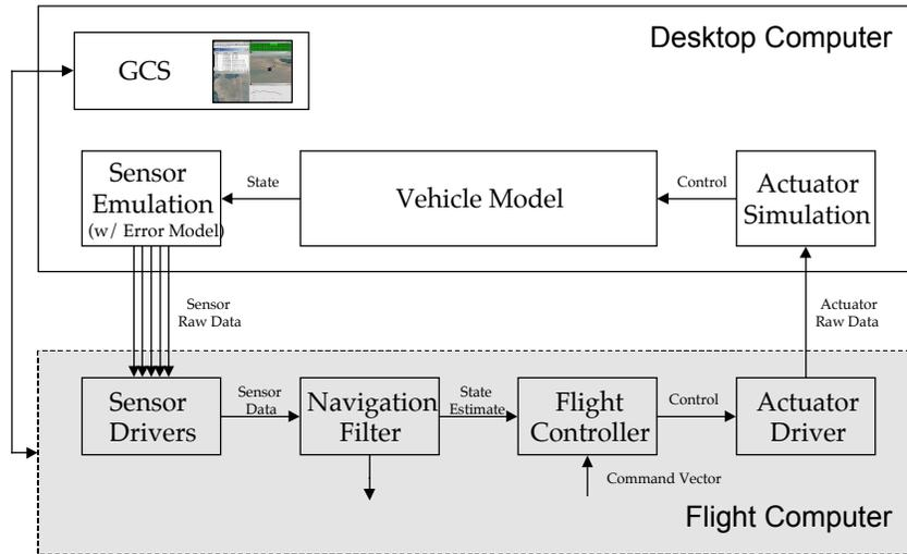
Fig. 6 Hardware in the loop structure for testing changes to the primary flight computer software or hardware.
