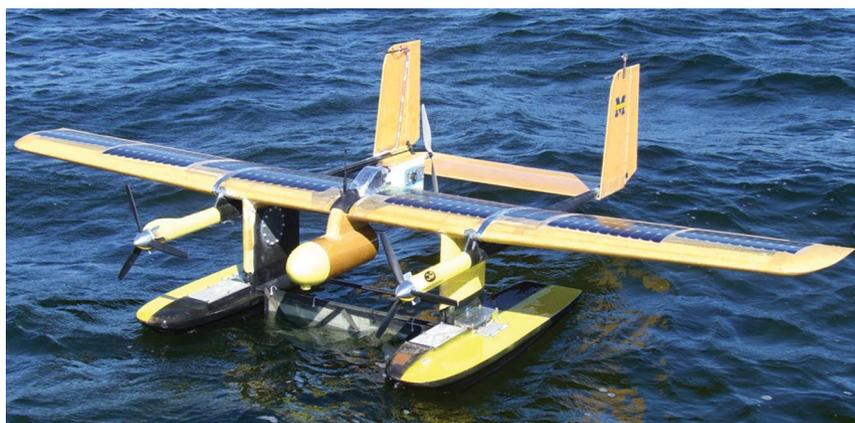
Fig. A1 Flying fish solar energy-harvesting autonomous seaplane (phase 2).
