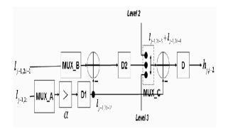
Fig. 3: Predict module of (5,3) filter
