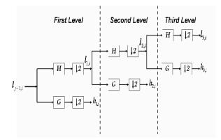
Fig. 1: Three-level analysis DWT
