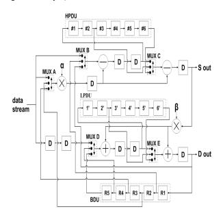
Fig. 5: Architecture of (5,3) wavelet transform
