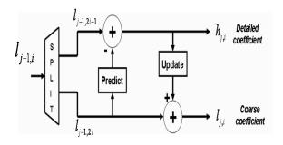
Fig. 2: Lifting DWT Module
