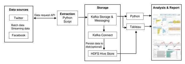
Fig.3 Stream Processing using Kafka – High-level Architecture and Process Flow
