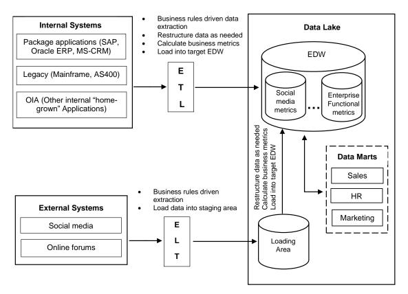
Fig.2 EDW built using ETL and ELT processes
