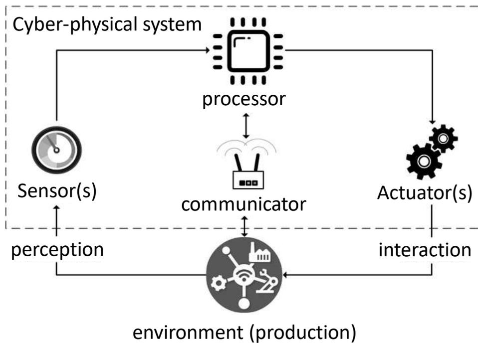
Figure 1: Schematic structure of a CPS
