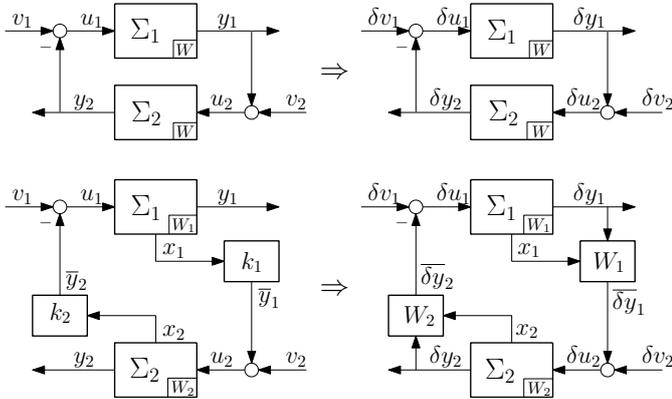
Fig. 2. Interconnection of uniform differential passive systems (top). Interconnection of differential passive systems (bottom).  $k_1(x_1)$  and  $k_2(x)$  define an interconnection on (15) that induces on the displacement dynamics (16) the cancellation  $-\delta y_1^T W_1(x_1) W_2(x_2) \delta y_2 + \delta y_2^T W_2(x_2) W_1(x_1) \delta y_1 = 0$ . They also define new output functions  $\delta y_i$  that guarantee uniform differential passivity.
