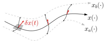
Fig. 1. The tangent vector  $\delta x(t)$  represents an infinitesimal variation on  $x(t)$ . Given an input curve  $u(\cdot)$  and its infinitesimal variation  $\delta u(\cdot)$ , the time-evolution of  $\delta x(\cdot)$  along a given solution  $x(\cdot)$  to (1) must satisfy (2). A precise characterization is given in Remark 1.
