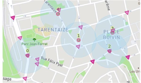
Fig. 1. A sample AVFAP problem instance, with demand sources (triangles) and taxis (circles) with their respective communication ranges (in blue).
