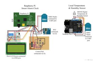
Fig. 5. Connection diagrams of the smart alarm clock.
