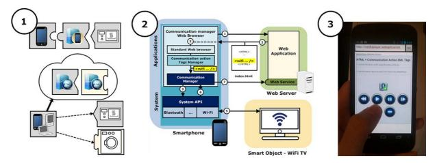
Fig. 1. (1) The solution is based on the use of distributed applications to interact with other devices and smart objects. (2) Communication Manager Web browser – Web Applications Scheme. (3) Image of a prototype web application used to control a media center.
