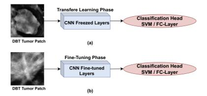
Figure 2. Feature extraction approaches: (a) transfere learning, and (b) fine-tuning.
