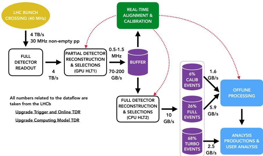
**Figure 2.** Scheme of the Real Time Analysis System. Data are first analysed in a GPU-based system called Allen, then buffered and finally reconstructed. The events with potentially interesting features are stored while the rest are discarded [5]
