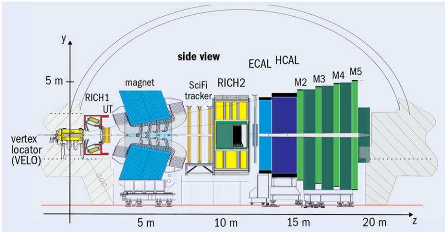
**Figure 1.** Layout of the LHCb detector. The detector elements, in order are the Vertex Locator, the first Cherenkov Radiation Imaging Chamber, the upstream tracker, the magnet, the scintillator fiber tracker, the second Cherenkov Radiation Imaging Chamber, the electromagnetic calorimeter, the hadronic calorimeter and the muon chambers.
