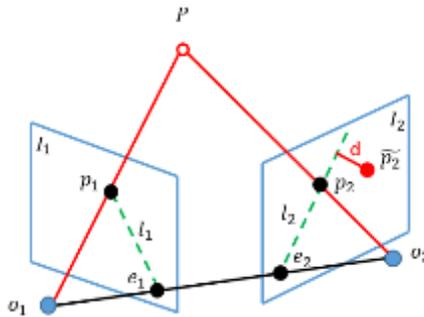
Figure 2. Schematic diagram of joint point matching based on epipolar constraint relation
