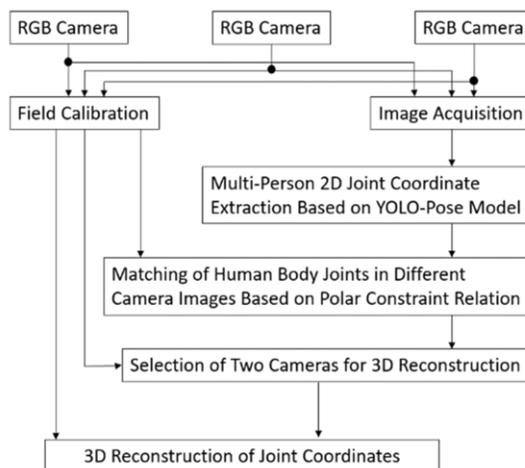
**Figure 1.** Function module of operation and maintenance personnel positioning and 3D joint point data acquisition system based on the multi-view stereo.
