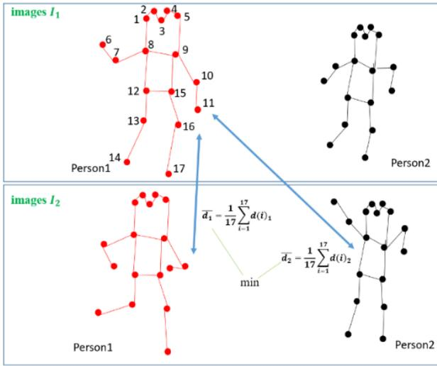
Figure 3. The schematic diagram of people matching principle
