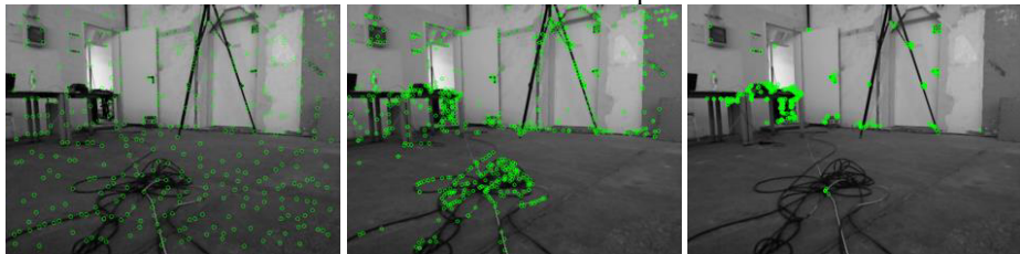
Figure 4. Effectiveness of different methods of feature extraction in low texture environments. HGCN(left), SIFT(middle), ORB(right)
