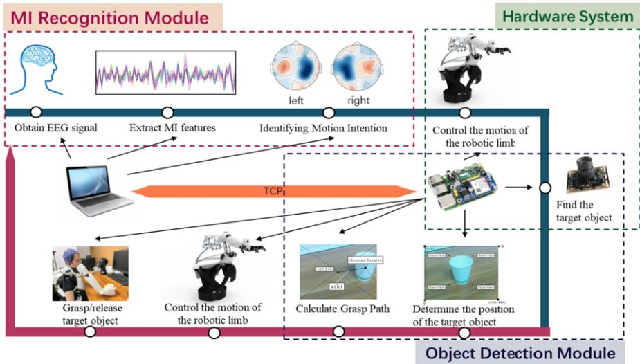
Figure 1. System framework diagram.
