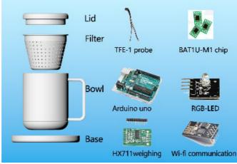
Figure 4. Tip Cup's hardware teacup and sensor.
