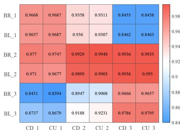
Fig. 13. Correlation coefficient of strain measurements from the experimental specimen.
