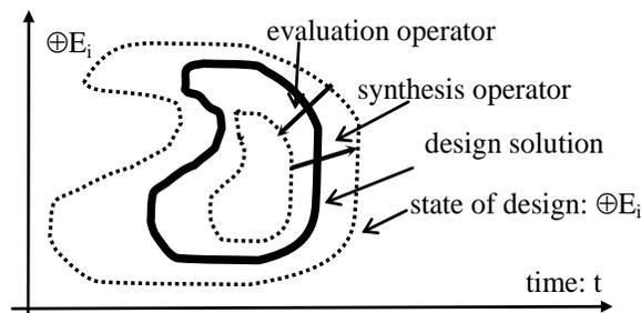
Fig. 4. State space of design under synthesis and evaluation operators (Zeng, 2004).
