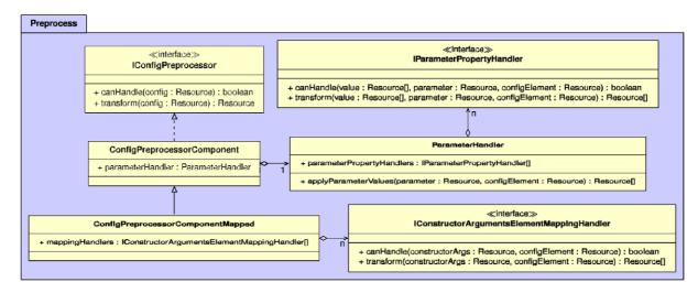
Fig. 5. UML diagram of the classes within the preprocess package, which are responsible for preprocessing config parameters and constructor arguments.
