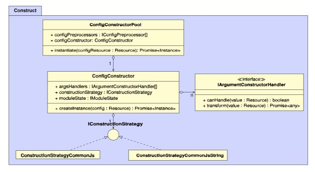
Fig. 6. UML diagram of the classes within the construct package, which are responsible for instantiating configs according to a certain strategy.
