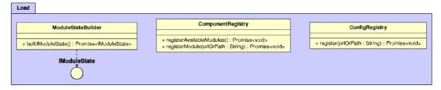
Fig. 4. UML diagram of the classes within the load package, which are responsible for loading components and configurations.
