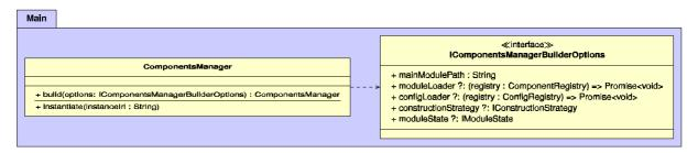
Fig. 3. UML diagram of the classes within the main package, which contains the main entrypoint of the framework.
