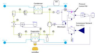
**Figure 10.** The refrigeration cycle is physically modelled. At this level the speed of the compressor is controlled either by the demand from the heat pump controller, or a PID which stops the system pressure getting too high.
