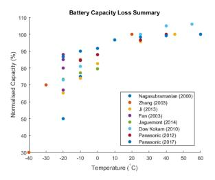
**Figure 1.** A summary of the capacity loss a function of temperature as reported by the following sources; Nagasubramanian (Nagasubramanian, 2001), Zhang (Zhang et al., 2003), Ji (Ji et al., 2013), Jaguemont (Jaguemont et al., 2014), Dow Kokam (Dow, 2010) (manufacturer) and Panasonic (Pan, 2012) (manufacturer).
