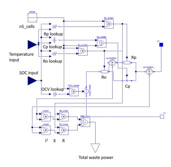
**Figure 3.** Electric first order RC model for the battery, scaled by number of cells in series using parameter nS\_cells, seen in the top right.
