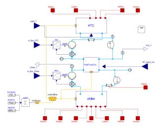
**Figure 7.** The middle level of the model contains the coolant circuits and the refrigeration loop and is used to control coolant flow between them.
