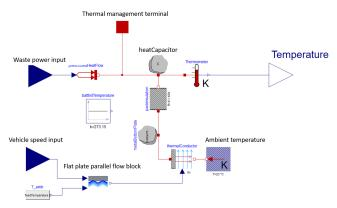
**Figure 4.** Thermal model of the battery with heat exchanges between ambient through a resistor to an exterior metal plate, and to the thermal management system through heat port seen at the top of the figure.
