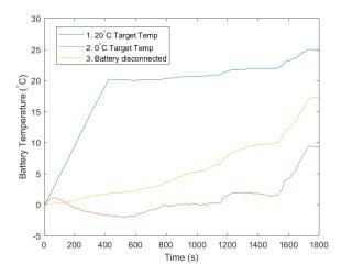
**Figure 12.** The battery temperature through the WLTP cycle shown for the first 3 scenarios proposed in case 1.
