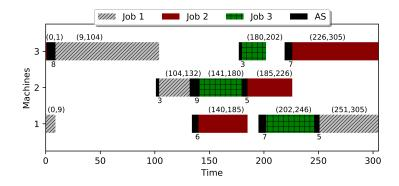
**Figure 6.** The detailed Gantt chart of the optimal solution found for the instance problem; blocking CJSS problem with sequence-dependent anticipatory setups (AS).
