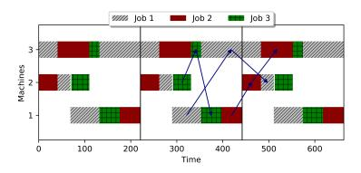
**Figure 5.** The Gantt chart of three consecutive cycles for the problem instance in Table 1; blocking CJSS problem.
