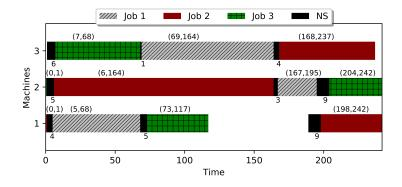
**Figure 8.** The detailed Gantt chart of the optimal solution found for the instance problem; blocking CJSS problem with sequence-dependent nonanticipatory setups (NS).
