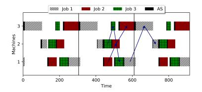
**Figure 7.** The Gantt chart of three consecutive cycles for the considered instance problem; blocking CJSS problem with sequence-dependent anticipatory setups (AS).
