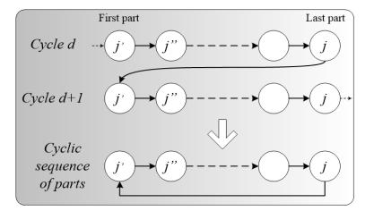
Figure 10. The cyclic sequence of parts on any machine.
