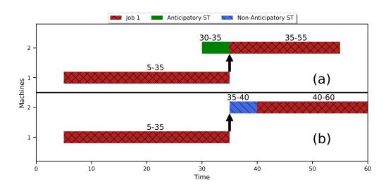
Figure 2. The anticipatory (a) and nonanticipatory (b) setups to process a job on a machine.
