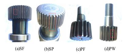
Figure 11. Gear fault feature diagrams.
