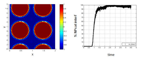
Figure 17. Percentage of NPs belonging to the interfacial region, in the absence of shear.
