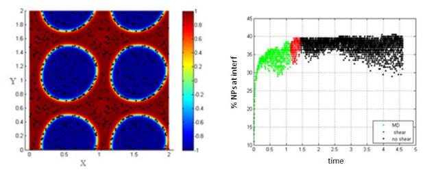
**Figure 5.** Shape deformation of the two fluids under the effect of shear (**left**); percentage of NPs belonging to the interfacial region in the regions, before applying shear (green), during applying shear (red), and after stopping shearing (black), Pe = 0.008 (**right**).
