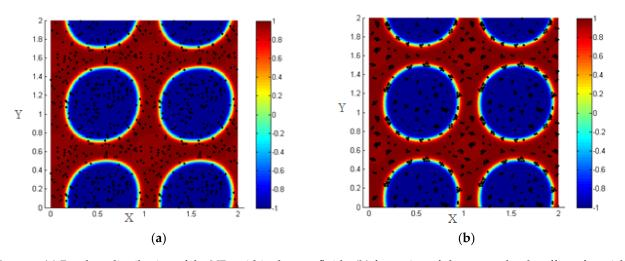
**Figure 8.** (a) Random distribution of the NPs within the two fluids; (b) formation of clusters under the effect of particleparticle interactions.
