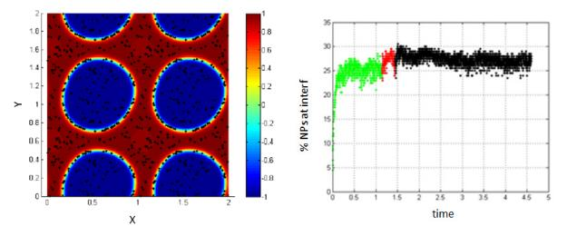
**Figure 10.** NPs near the interface migrate to the interfacial region (**left**); percentage of NPs belonging to the interfacial region in the regions, before applying shear (green), during applying shear (red) and after stopping shearing (black), Pe = 0.008 (**right**).
