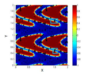
Figure 12. Some clusters are attached between two adjacent interfaces, *Pe* = 0.316.
