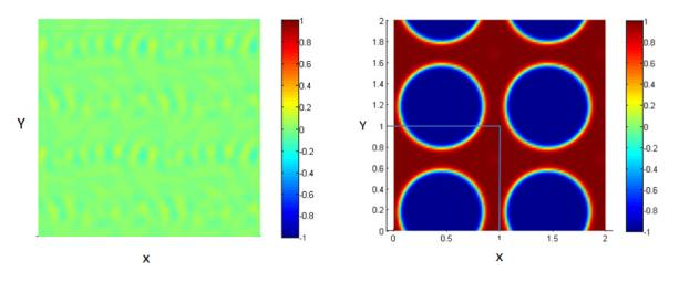
**Figure 2.** Mixture of two immiscible liquids, from the homogenous state (**left**) to the equilibrium state after the phase separation (**right**).
