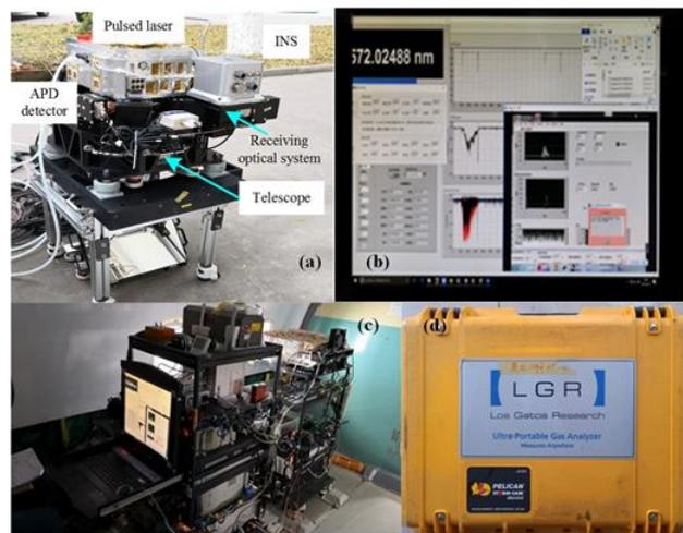
**Figure 3.** Photographs of the IPDA LIDAR system. (a) The transceiver system mounted in a pod outside the aircraft. (b) The control interfaces of some instruments. (c) The environmental control, control electronics, seeder laser and frequency stabilization system are installed inside the aircraft. (d) The in-situ instrument for CO<sub>2</sub> measurement is mounted inside the aircraft.
