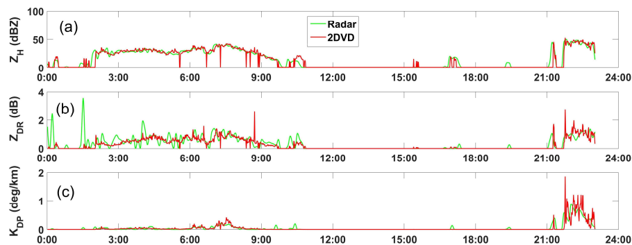
Figure 7. The time-series comparison of radar moments simulated by raindrop size distribution (DSD) data with T -matrix method and measured polarimetric parameters during Super Typhoon Hato: (a) Z_H , (b) Z_{DR} , (c) K_{DP} .
