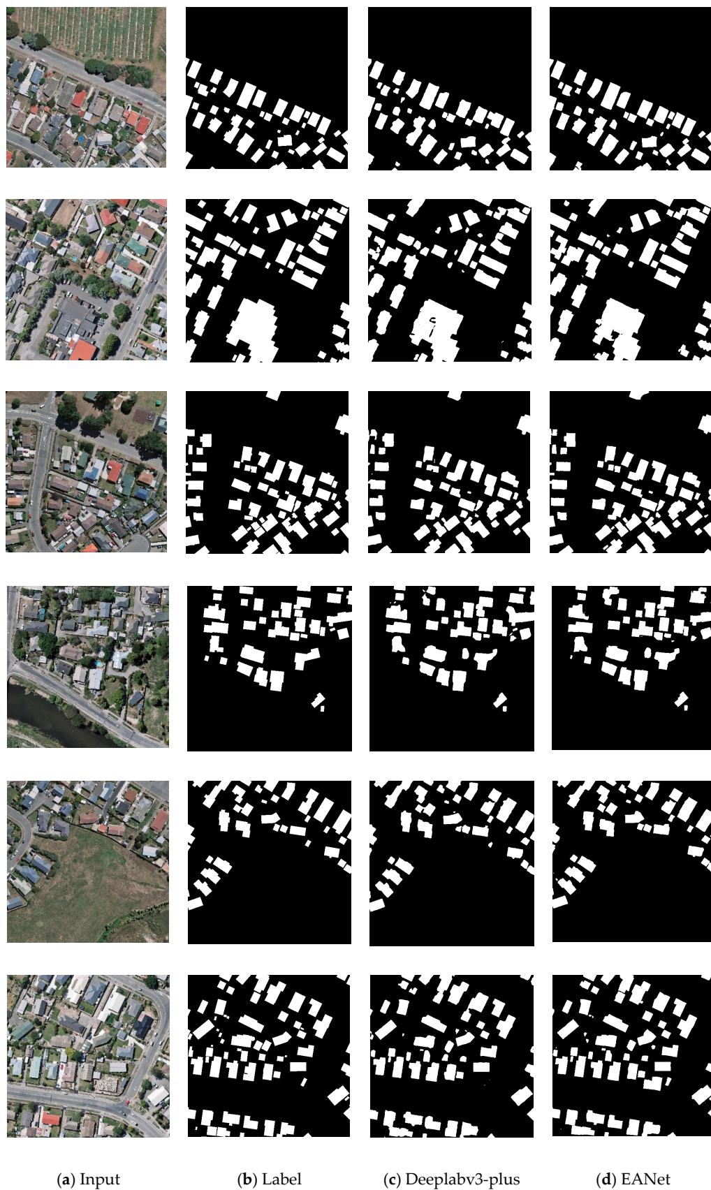
Figure 7. Experimental results with the Wuhan University (WHU) building validation set. (a) Original image selected from the dataset. (b) Image label. (c) BiSeNet processing result. (d) EANet processing result.
