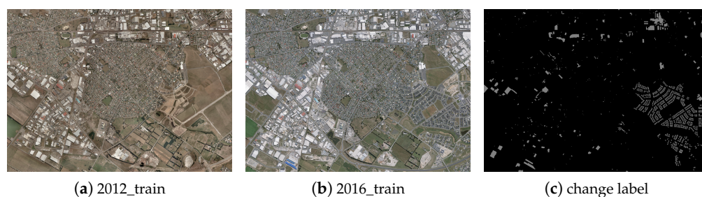
Figure 4. The WHU change detection dataset. (a) is the whole training image of 2012 of the WHU change detection dataset, which is used as the source domain in our experiment; (b) is the whole training image of 2016 of the WHU change detection dataset, which is used as the target domain in our experiment; (c) is the ground-truth for the change in the WHU change detection dataset.
