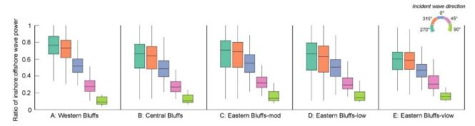
**Figure 10.** Ratio of inshore to offshore wave power along five distinct sections of Barter Island as a function of offshore incident wave directions. WB, EB, and CB denote the western, eastern, and central bluffs, respectively. Eastern bluff sections are further divided by moderate to very low bluff recession rates (see Figure 7a). Ratios were computed from wave model runs of 2000 individual events of varying wind and offshore wave conditions.
