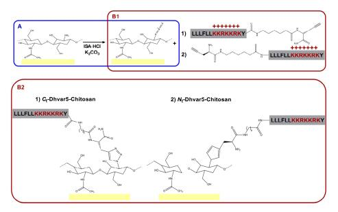
**Figure 1.** (**A**) Chitosan functionalization by direct conversion of the amines in the chitosan ultrathin film coatings into azides ( $N_3$ -chitosan); (**B1**) CuAAC "click" reaction between the azide group on  $N_3$ -chitosan and the alkyne group in the Pra residue inserted at either the peptide's (**1**) C-terminus or (**2**) N-terminus, to originate (**B2**) the Dhvar5-grafted chitosan films (**1**)  $C_t$ -Dhvar5-Chitosan and (**2**)  $N_t$ -Dhvar5-Chitosan.
