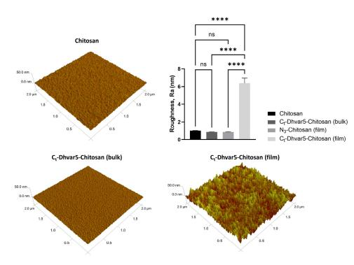
**Figure 6.** Atomic force microscopy (AFM) micrographs to evaluate surface topography and respective roughness (Ra) quantification (One-way ANOVA, \*\*\*\* p < 0.0001); data represent mean  $\pm$  standard deviation; ns: non-significant.
