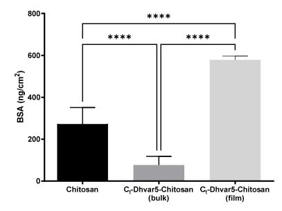
**Figure 8.** Adsorption of BSA (4 mg/mL solution in PBS, injected in the system at a flow rate of 25  $\mu$ L/min) onto unmodified and peptide-modified chitosan films before and after film fabrication (Kruskal–Wallis test, \*\*\*\* *p* < 0.0001); data represent mean  $\pm$  standard deviation.
