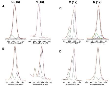
**Figure 5.** XPS high-resolution spectra of (**A**) unmodified chitosan, (**B**)  $N_3$ -chitosan, (**C**)  $C_t$ -Dhvar5-Chitosan, and (**D**)  $N_t$ -Dhvar5-Chitosan, for *C1s* and *N1s* regions.
