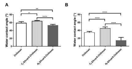
**Figure 3.** WCA for chitosan and chitosan-functionalized films determined by (**A**) sessile drop and (**B**) captive bubble methods (One-Way ANOVA analysis, \*\* p < 0.004, \*\*\*\* p < 0.0001); data represent mean  $\pm$  standard deviation.
