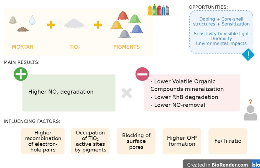
**Figure 2.** The interaction of pigments and TiO<sub>2</sub> in mortars: main findings and opportunities based on the literature review.
