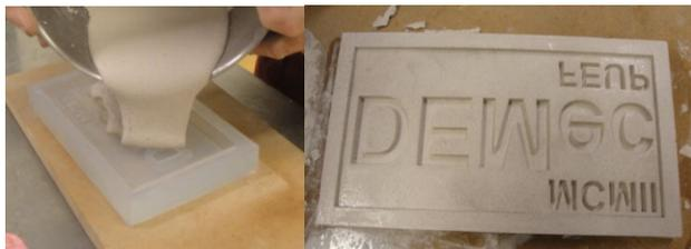
Figure 10. Casting the ceramic slurry and final ceramic mould.
