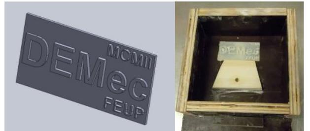
Figure 7. Image of the metallic plate to be obtained and SL prototype with the gating system.
