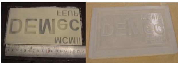
Figure 9. Stereolithography model and silicon mould.
