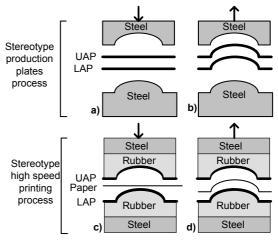
Figure 4. The stereotype production scheme.
