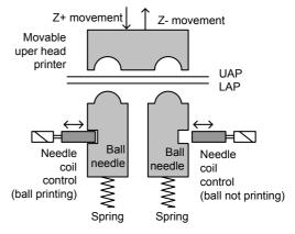
Figure 9. The printer head.
