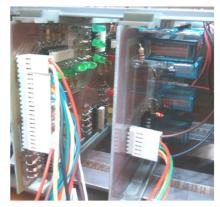
Figure 12. The electronic box with the new PCBs installed.
