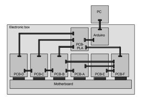
Figure 11. The new PCBs scheme on the electronic box and the PC connection.
