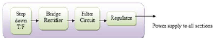
Fig. 3. Block Diagram of Power Supply
