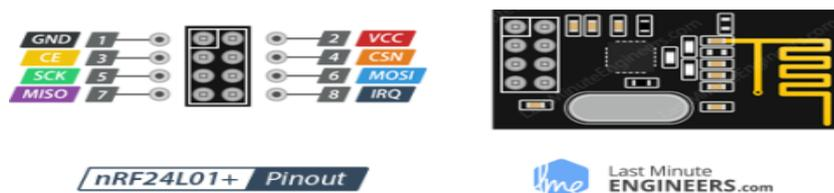
Fig. 6. Pinout of nRF24L01
