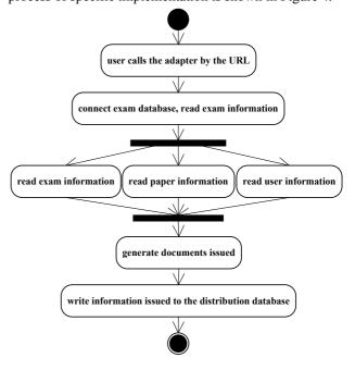
Figure 4.The program flowchart of adapter
