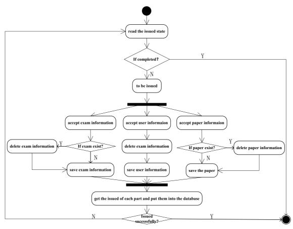
Figure 5. The program flowchart of data distribution
