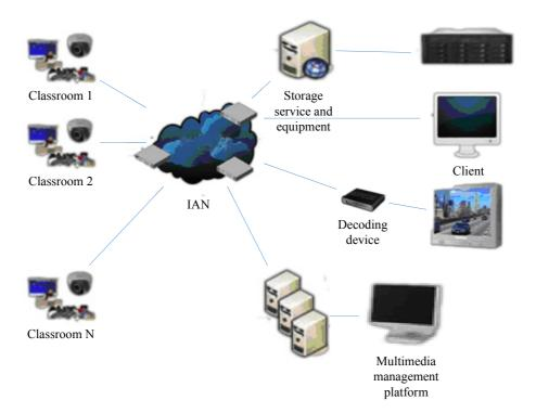
Fig. 5. Structure of the system
