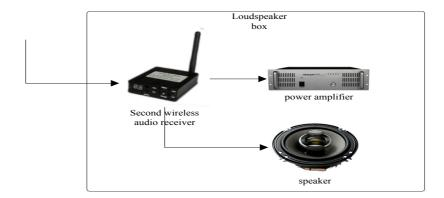
Fig. 4. Structure of the speaker
