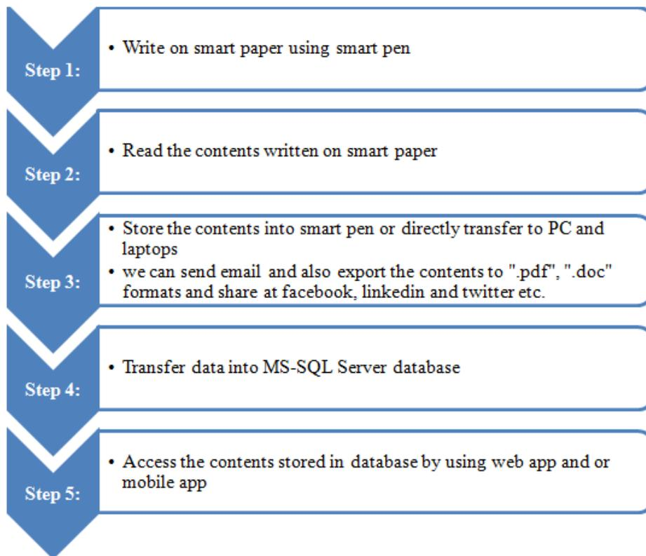
Step 1 is to write on the smart paper by using smart pen which has the features of digital capturing, transmission and processing of data and drawings figures on paper.
